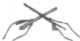
Fig. (i): Making a scratch on the glass tube
