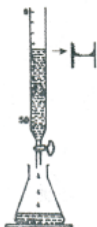
Fig. 15.1: Correct way to note down the burette readings
