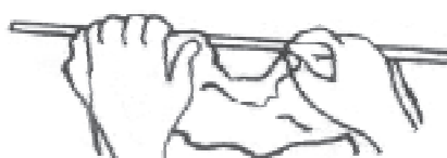
Fig. (ii): Holding & Breaking a glass tube
